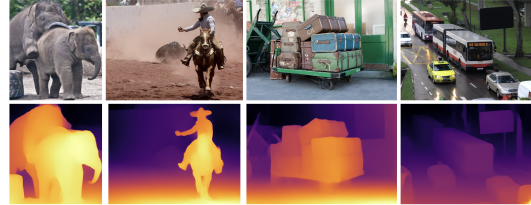
Figure 4. Outputs of running MiDaS depth estimation model on a random subset of single-view input images. Figure taken from Ranftl et al. [10]
