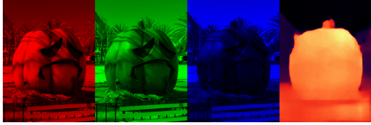
Figure 12. RGB-D image channels, where the depth channel is predicted by the Tiefenrausch method
